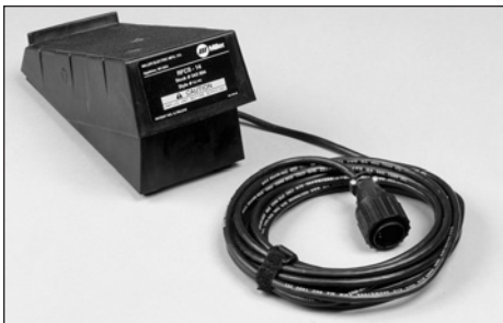
Figure 3.26 TIG foot control. A foot-operated remote output and current control.
