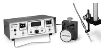
Figure 3.38 A seam tracker for maintaining the arc and joint alignment.
