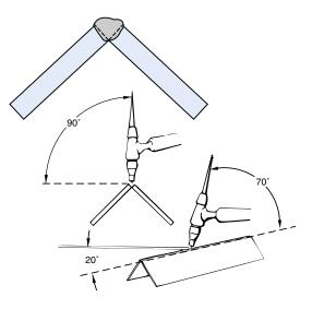
Figure 8.8 Welding the corner joint.
