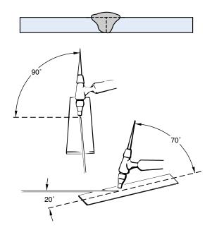
Figure 8.5 Welding the butt weld and stringer bead.
