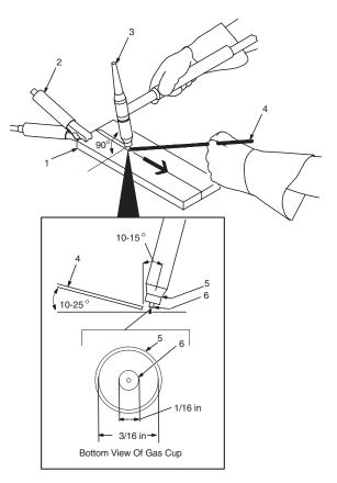
Figure 8.2 Gas cup size and torch positions. 1-Workpiece, 2-Work Clamp, 3-Torch, 4-Filler Rod (If Applicable), 5-Gas Cup, 6-Tungsten Electrode.
