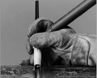
Figures 8.11 and 8.12 Demonstrations of two common methods of grasping the torch for pipe welding. There is no single "correct" method of doing this and each welder is encouraged to experiment with several different methods until one is found that is most comfortable, and results in satisfactory welds.
