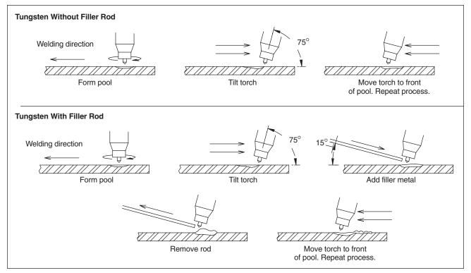
Figure 8.4 Torch movement during welding.
