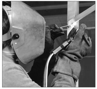
Figure 8.10 Welding in the overhead position.
