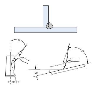
Figure 8.7 Welding the T-joint.
