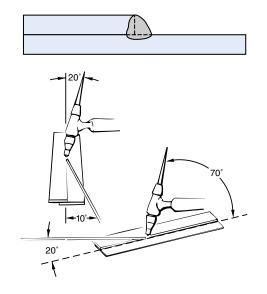
Figure 8.6 Welding the lap joint.
