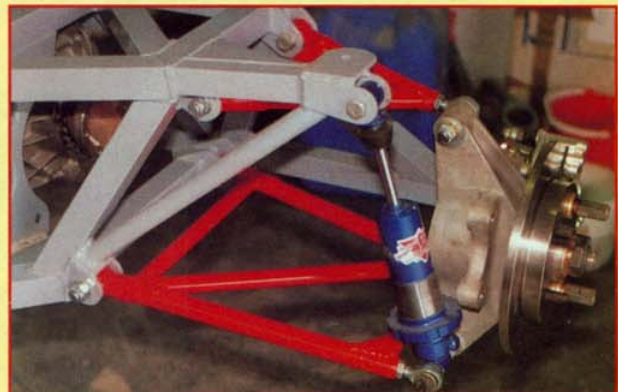
The rear suspension uses 1" and 3/4" CDS round tube wishbones with cast aluminium uprights. Differential including LSD option, driveshafts, hubs and brakes are Ford Scorpio.
