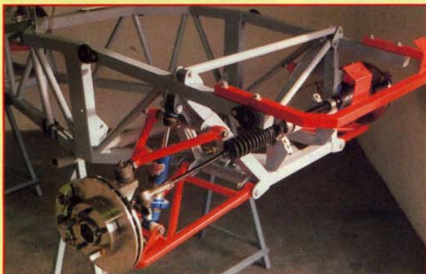
Euro chassis front suspension uses 1" and 3/4" CDS round tube wishbones allied to cast aluminium uprights with Ford Scorpio hubs and brakes. The detachable front frame carries the radiator.
