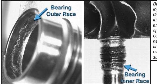
Ball bearing races damaged by intense heat and high turbo speeds. The ball bearings had a tough time rolling over these surfaces!
