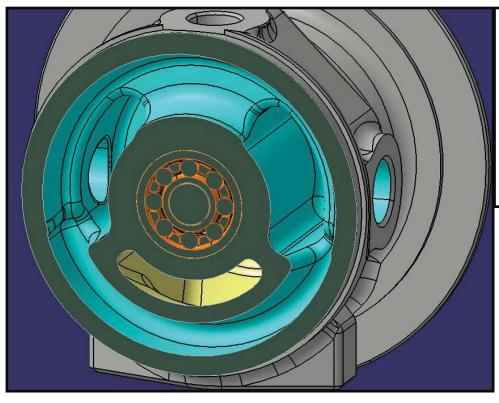
Turbo center housing shown in cutaway view, with water cavity (blue), oil cavity (yellow). Water cavity completely surrounds ball bearing cartridge (orange) and has a port on either side for water inlet & outlet.
