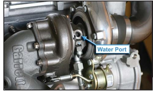
Water cooling's main benefit actually occurs after the engine has been shut down. Heat
