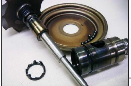
Overheated ball bearing cartridge, disassembled showing damaged retainer at lower left. Bearing races are blued and damaged as well. Excessive play is the result of retainer and race damage, often culminating in wheelto-housing rubbing and total turbo failure.
