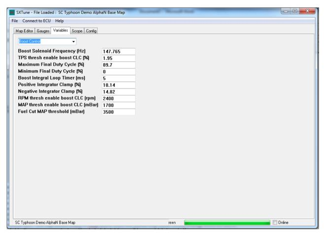
This Boost Control page displays values relating to the closed loop boost control strategy and is broken down into:
