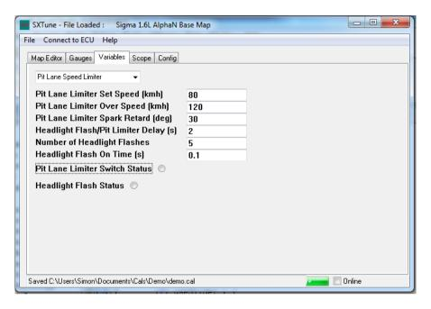
The Pit Lane Speed Limiter is used to control the maximum vehicle speed to a set value when the ECU pit lane speed limiter switch is enabled. The values required to calibrate the pit lane speed limiter function are in the 'Pit Lane Speed Limiter' variables page.
