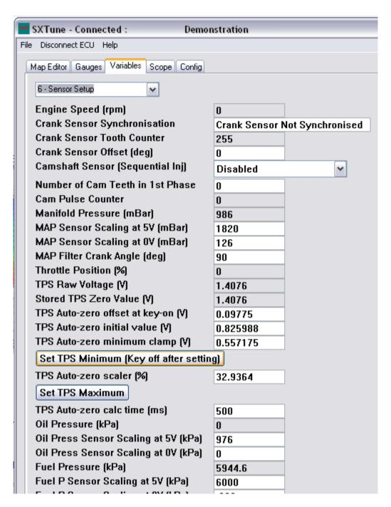
To calibrate the throttle position sensor click the 'Variables' tab and select option 6 "Sensor Setup" from the drop down.
