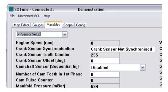
Set the 'Camshaft Sensor' drop down to 'Disabled' then crank the engine over with the ignition coil and fuel pump relay disconnected. You will see the 'Crank Tooth Counter' increment as each crank tooth passes the sensor. When the ECU sees the correct number of teeth followed by either the correct number of additional tooth/teeth or missing tooth/teeth then the Synchronisation will switch from 'Not Synchronised' to 'Crank Sensor Synchronised OK'.
