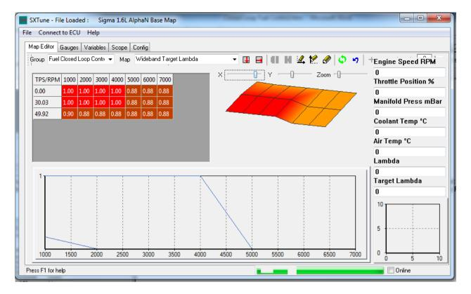
The Wideband Target Lambda map is located in the 'Fuel Closed Loop Control' Group and should be calibrated to the desired lambda for the engine. Typically a normally aspirated engine will run at Lambda 1.00 at part load, low speed and 0.85-0.88 at full load to achieve maximum power. Turbocharged engines will need to run richer than this to reduce exhaust gas temperatures.
