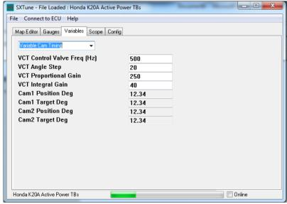
This page contains variables relating to the variable valve timing control strategy. It is broken down into:
