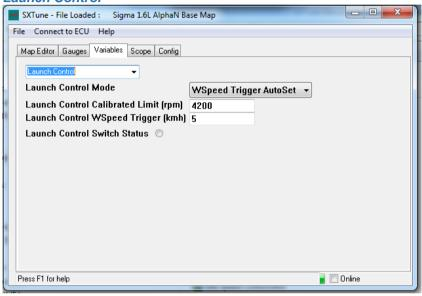
Typhoon and Tornado feature a launch control strategy to optimise acceleration from a standing start. This function operates by holding a set engine speed regardless of throttle position when stationary, this limiter is cancelled when the vehicle starts to move allowing the engine speed to increase.
