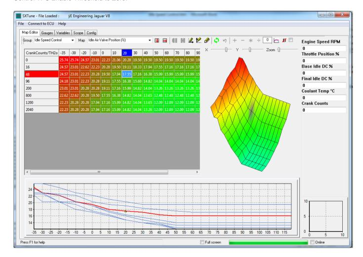
**N.B.** For electronic throttle applications Idle Air Valve duty cycle is translated directly into a throttle position value by dividing the final duty cycle by 4. This percentage value is added directly to the target TPS % for idle speed air control. For clarity, from this point onwards this guide will refer only to Idle Air Valve position.
