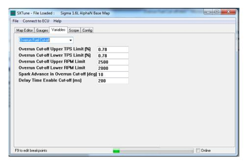
This page contains variables relating to the over-run fuel cut off strategy and is broken down into:
