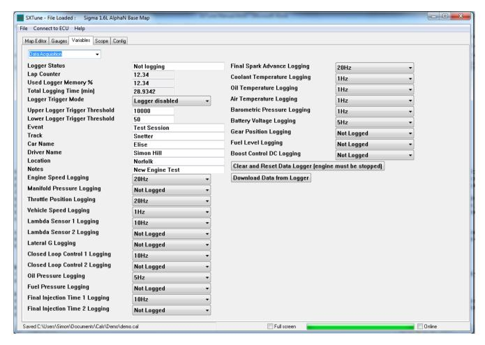
Tornado 2 and Typhoon 2 are supplied with an internal data acquisition system that can log channels up to 100Hz. Data is stored in the ECU and downloaded after each session to be viewed in the SXLogView data analysis program. It is configured and controlled directly from the 'Data Acquisition' variables page, as described below:
