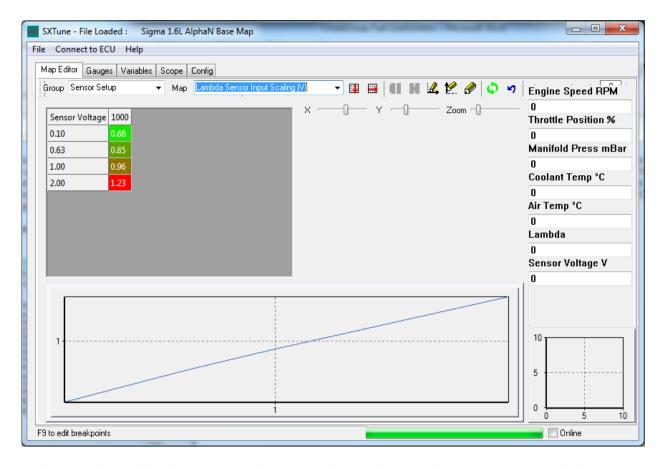
Before enabling wideband sensor control the sensor input voltage scaling must be entered. In the Map Editor, Group - 'Sensor Setup', Map - 'Lambda Sensor Input Scaling (V)' the output voltage of the chosen wideband lambda controller vs lambda can be entered. This is a variable breakpoint map, voltage breakpoints can be entered using F9, to return to the map press F11.
