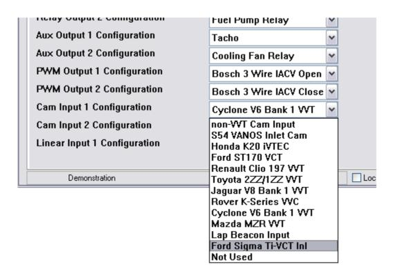
Trigger patterns for both Cam Inputs 1 & 2 can be selected in 'Variables' tab option '2 – ECU Configuration'. A wide range of original equipment camshaft triggers can be accommodated to enable variable valve timing control. For a conventional non varying camshaft input select the option 'non-VVT Cam Input'. Then enter the number of cam teeth pulses in the first phase (Cylinder #1 firing) into 'Variables' option '6 – Sensor Setup'.
