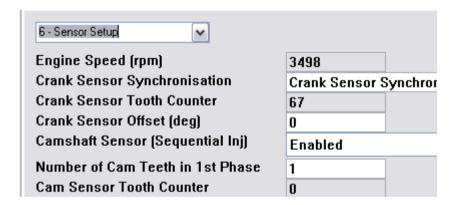
Enable the camshaft trigger by selecting 'Enabled' in the Camshaft Sensor drop down. This will also enable sequential injection. If this option is disabled, the ECU will still inject once pulse per cycle, but this could either be in either phase.
