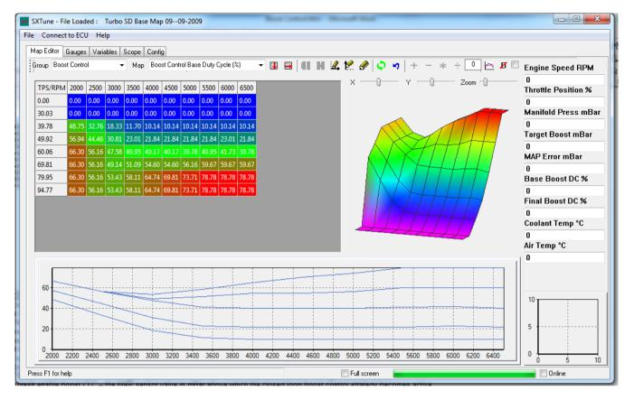
The open loop boost control term is calculated by a map as a function of throttle position and engine speed. This should be calibrated to achieve the target boost level before closed loop boost control is enabled. The target manifold pressure in mBar is calculated from a map also as a function of throttle position and speed.
