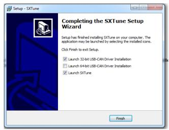
N.B. You MUST install the USB-CAN interface drivers onto your PC before plugging in the USB-CAN interface. If the drivers are not installed, SXTune will show the error message 'CAN Interface Not Found' when trying to connect. The USB-CAN drivers should be installed as part of the SXTune installation, but they can also be downloaded separately from the SC website: <a href="https://www.twinkam.co.uk">www.twinkam.co.uk</a>.
