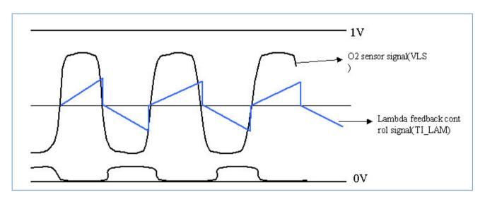
The proportional and integral step sizes are set by four maps as a function of throttle position and engine speed. The scope page is a useful tool in monitoring the closed loop control loop and determining the correct operation of the system. Ultimately the system performance can be measured by an exhaust gas analyser; the system should be optimised as a compromise between engine performance and tailpipe emissions.
