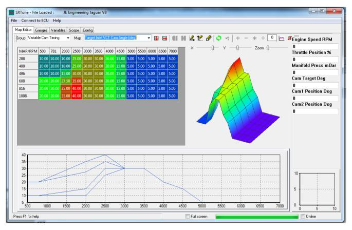
Typhoon and Tornado feature dual variable camshaft timing control. This can be used as either inlet and exhaust camshaft control on an inline engine or dual inlet camshaft control on a vee engine. Target camshaft position is calculated from a map of load (TPS or MAP) and engine speed. Closed loop control is achieved by means of a proportional-integral controller, the gains of which can be set in the 'Variable Cam Timing' variables page.
