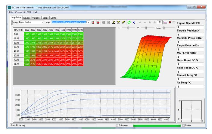
This forms the set point of the proportional-integral closed loop boost controller. The integral and proportional gain terms are set by maps as a function of the error between the target MAP (set point) and the actual measured MAP.
