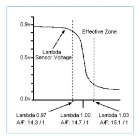
To promote the thermal reaction in a catalytic converter it is necessary to cycle the fuelling slightly rich and lean of Lambda 1.00. The resultant differences in oxygen content of the exhaust allow the catalyst to alternate between "oxidizing" CO and HC and "reducing" NOx.
