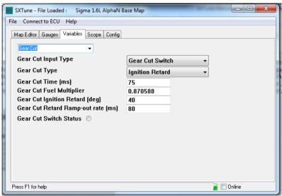
This page contains variables relating to the Gear Shift Cut Function:
