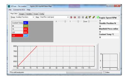
Rev limiting (over-speed protection) is implemented by a user selectable range of hard and soft cuts. The primary hard rev limit is set by a Map 'Hard Rev Limit (rpm)' under the Group 'Auxiliary Functions'. This map is a function of coolant temperature, enabling a reduced rev limit to be set when the engine is too hot or too cold providing increased engine protection.
